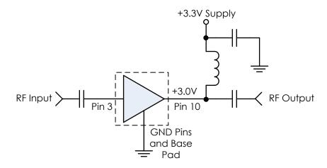
\*External DC blocking capacitors and RF choke are required. Select values for the frequency range of interest. No input or output matching is required. NC pins may be left open or connected to ground.
