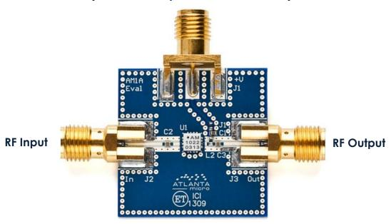
External DC blocking capacitors and RF choke are included.
